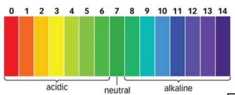
You can use universal indicator or a pH probe to measure the acidity or alkalinity of a solution against the pH scale.
