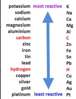
The ions discharged when an aqueous solution is electrolysed using inert electrodes depend on the relative reactivity of the elements involved.
