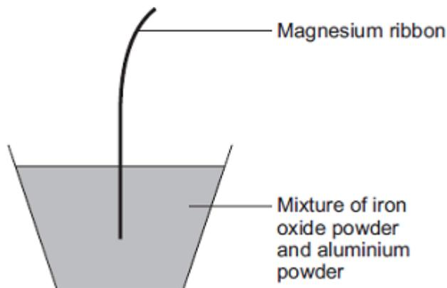
Iron oxide reacts with aluminium to produce iron.
