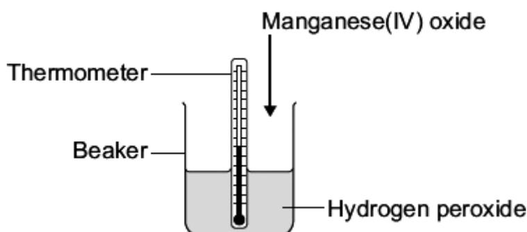
The student first measured the temperature of the hydrogen peroxide. Then the student added the manganese(IV) oxide, stirred the mixture and recorded the highest temperature.
